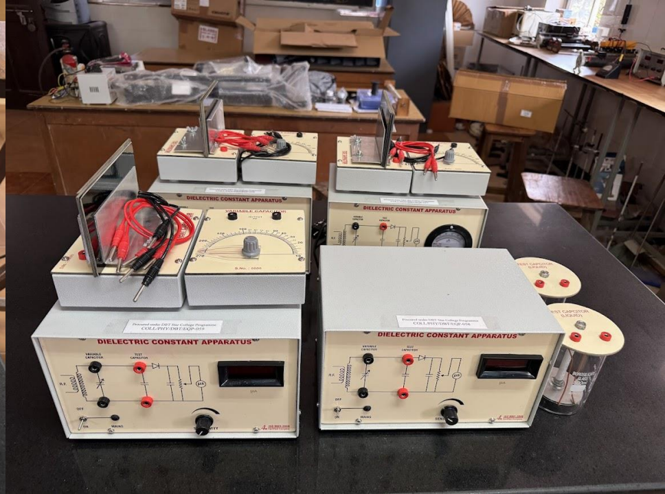
Dielectric Constant set up of Solids and Liquids
