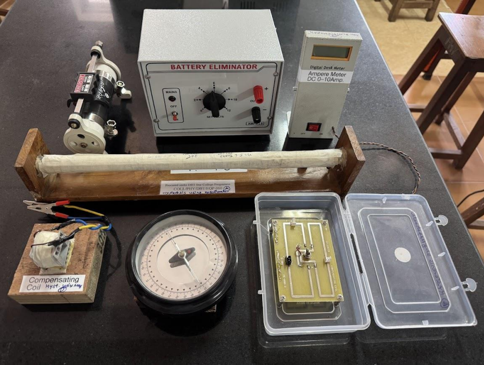
Experimental Setup to Find Hysteresis of Using Magnetometer
